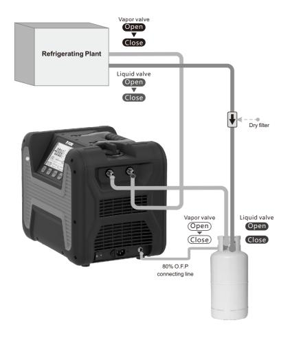
This method is only for larger systems with at least 14 kg of Liquid refrigerant. It's used to recover liquid before recovering vapor.
