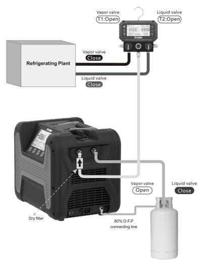
This is the typical recovery method. Vapor and liquid lines are routed through your manifold, into AR600, and out to the recovery cylinder. CAUTION: Understand all class A2L refrigerant warnings and notices if applicable (pages 1, 5).
