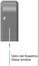
Place the gasket **(F)** against the top part of the window glass (taking into account what was mentioned previously), note and cut following the profile of the window itself.
