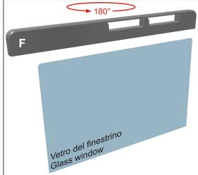
The bottom part of the gasket **(F)** is equipped with a groove along its entire length; this should be locked with the top part of the window glass.
