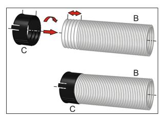
In order to connect the flexible tubing **(B)** of "CUBE" it is sufficient to click the nozzles' winglets **(C)** into the grooves of the various components.
