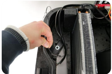
4) Disconnect the RT1 white connector from the main PCB and then remove the evaporator temperature sensor
