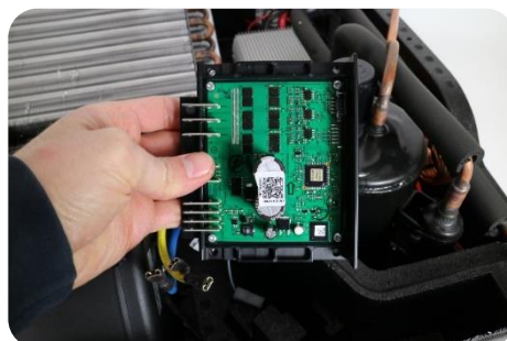
4) Disconnect all the wires from the PCB connectors and then remove the PCB with a new one
