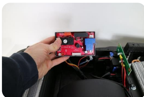
4) Disconnect all the connectors from the main PCB, remove the PCB and replace it with a new one
